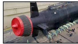
Propulsor Ducts Submarine
